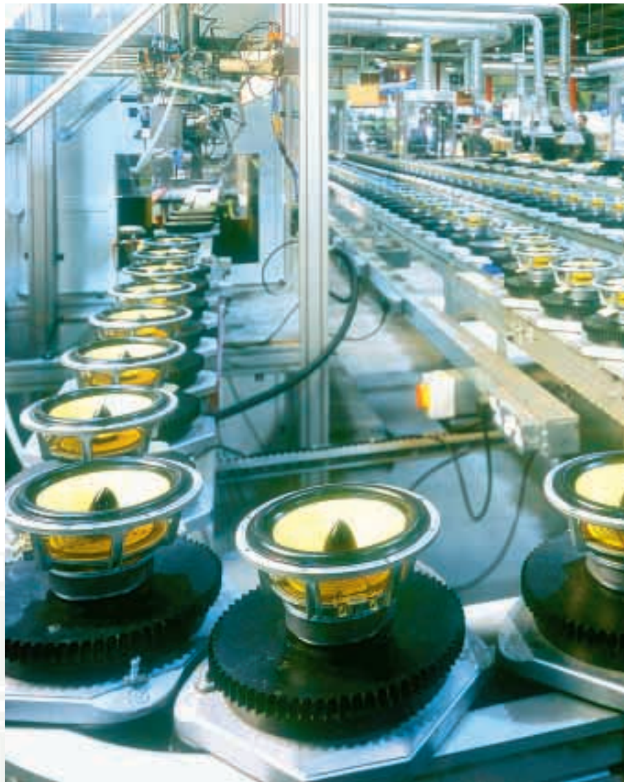
Satellite system for automatic gluing of loudspeaker bass unit elements.
