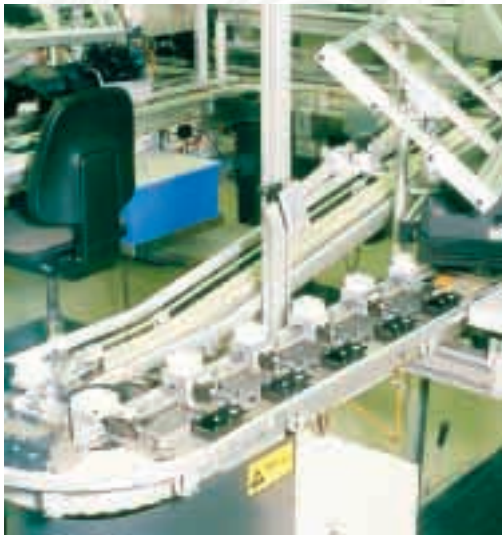
Pallet buffer in a manual working station for assembly of electrical shavers.
