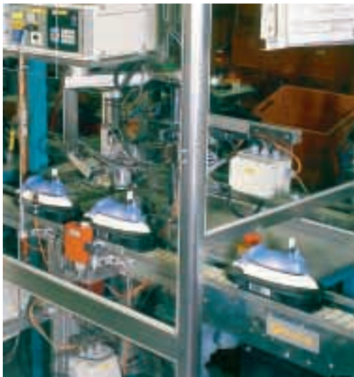
Fully automated test station with integrated pallet conveyor for steam irons.
