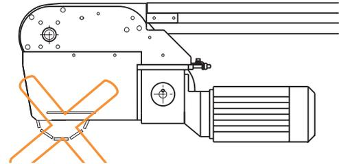
*Slack protection plate for drive unit type H*
