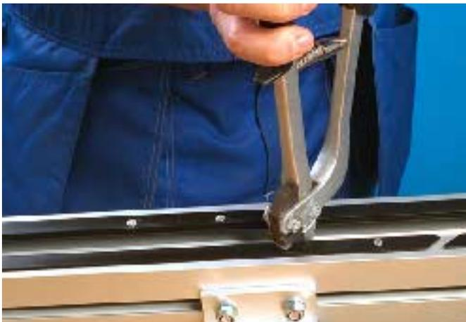
1 Insert rivets in the holes, using rivet crimping pliers or a rivet crimping clamp. For type of rivet, see table on previous page.
