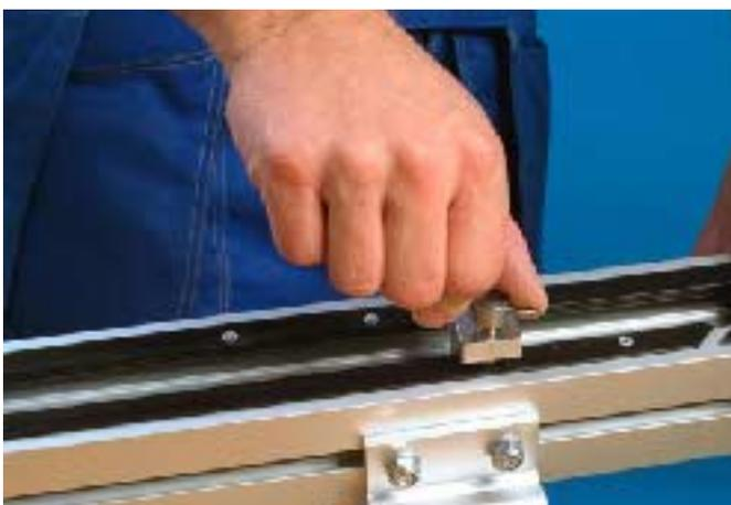
2 If working space is limited, the rivet crimping clamp might be easier to use. The two crimping tools perform the same task, but the pliers are more efficient and easier to use.
