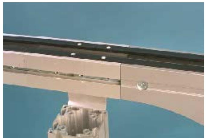
4 Keep a distance of approximately 30 mm between rivets and idler unit. This is in case the idler unit has to be removed after conveyor system assembly.
