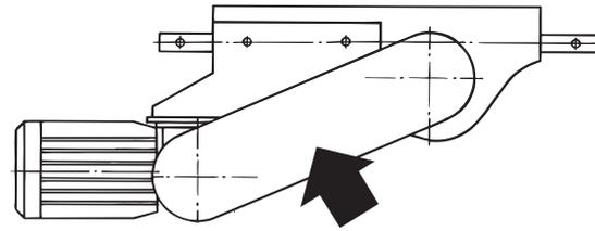
*Chain guard for roller chain transmission*
