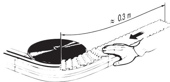
*Sample for checking conveyor chain space*
