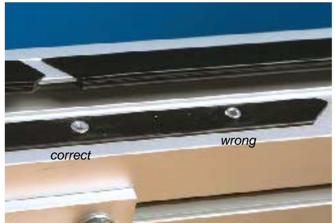
3 Check that the rivets do not protrude over the surface of the slide rail.
